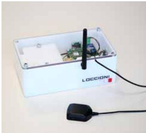
Wireless accelerometer node
